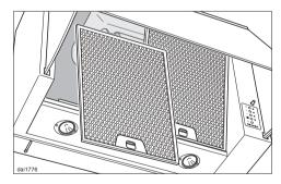
■ Finally, replace the grease filters.
